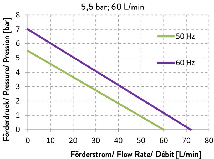
Fig. 104: IN 1030 T, IN 1330 TW, IN 1830 TW
